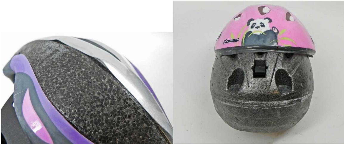
Damage to the helmet stickers and fitting foam was extensive. Some stickers came off in the initial washings, and most had come off when the tests were done. Fitting foam detached from the inside of the helmet liners in all cases, and some disintegrated .
