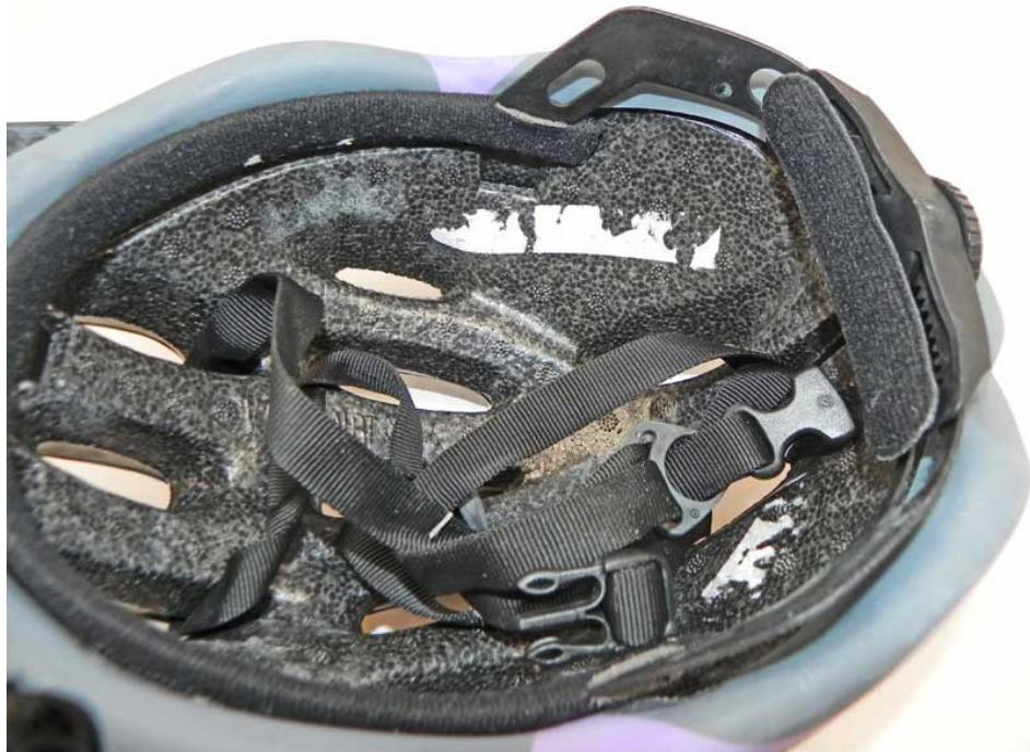
Since the stickers are essential to identifying the helmet and the standard the manufacturer certifies it to, we consider sticker loss as substantial damage. Fitting foam is required to keep the helmet in place for a crash, so losing it is critical to performance.
